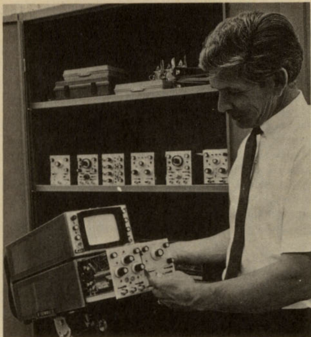
FIG 11-38 A high-frequency oscilloscope with plug-ins for both x and y axes. (Hewlett-Packard Company.)
