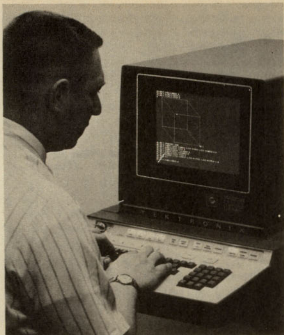
FIG 11-54 A computer terminal using a phosphor-storage CRT display. (Tektronix, Inc.)
