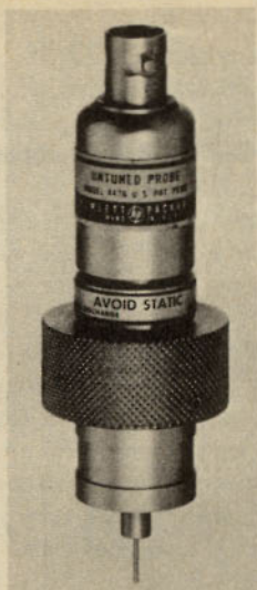
FIG 17-2 Slotted-line detector probe, Hewlett-Packard Company 447A.
